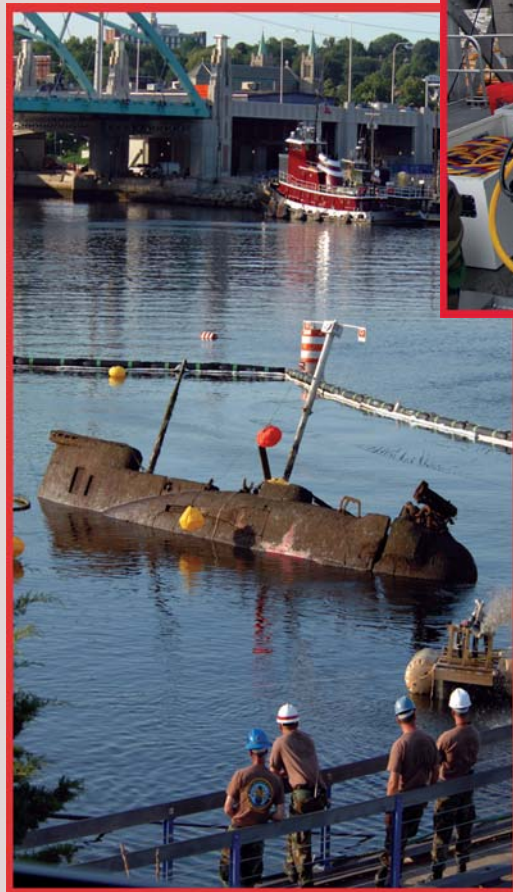
J-484's sail emerges as salvors right the sub with cable pullers.
